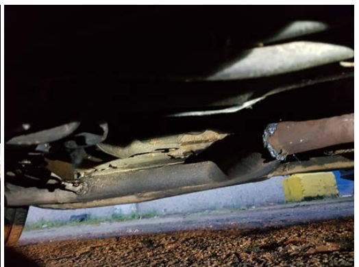
Removed catalytic converter from a German Opel Astra from 2000 (left picture) and from a German BMW 3181 from 1998 (right picture) © ILT December 2019
